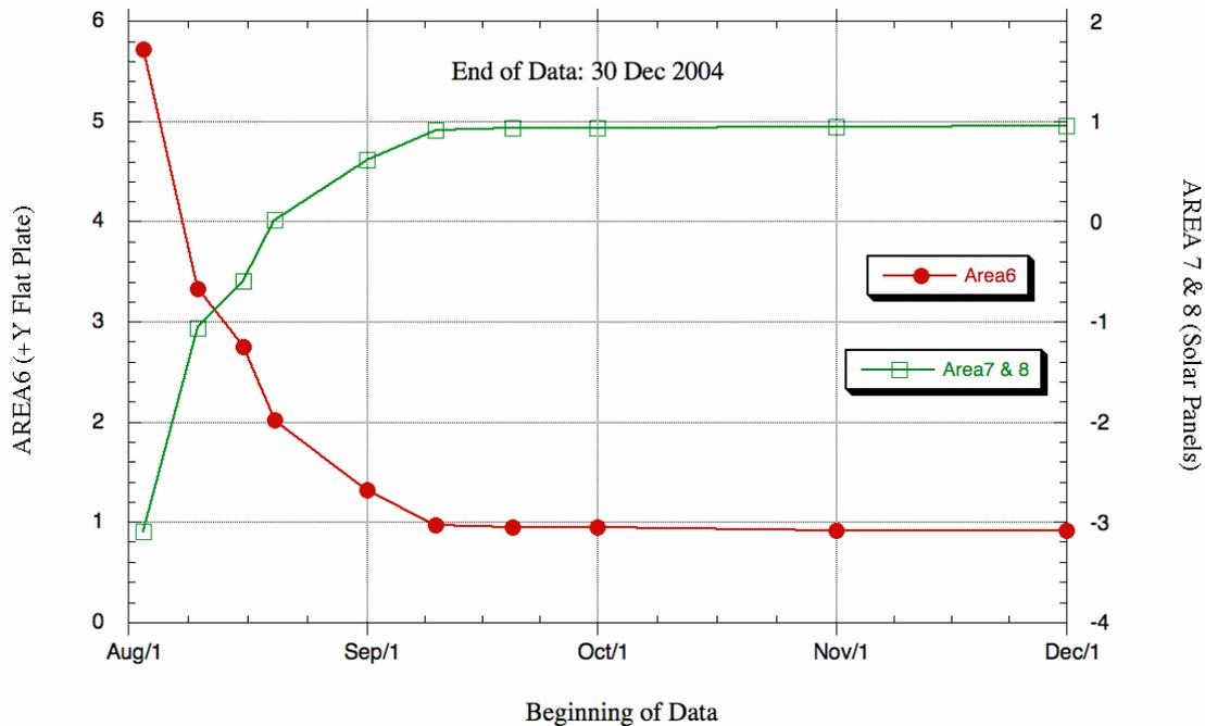
**Figure 2. Solar Radiation Pressure Scale Factor Estimates for Various Tracking Data Start Times Showing Stability of Estimates for Main Body (Area6) and Solar Panels (Area 7&8) After Early Data are Excluded.**
